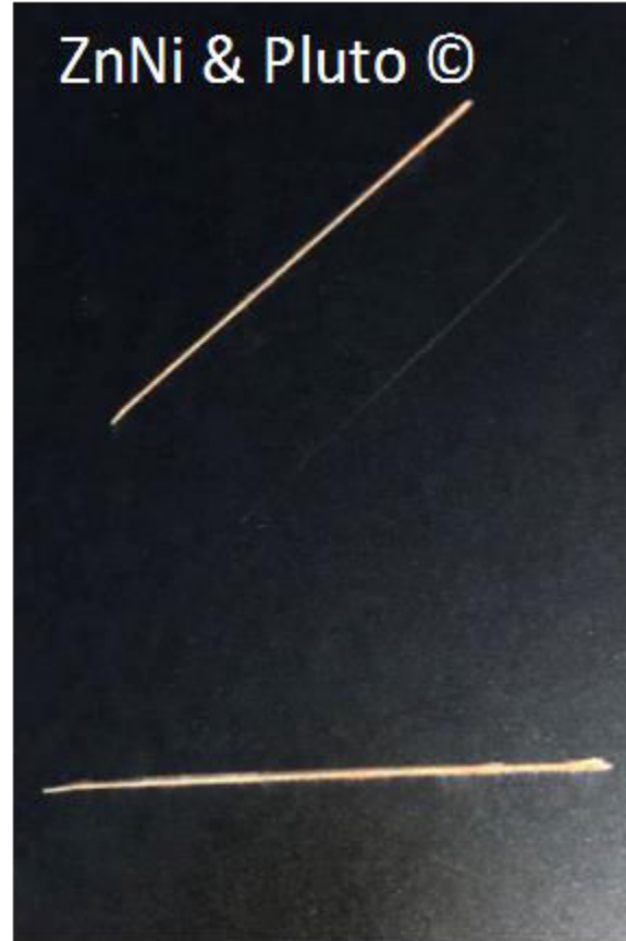
August 2018, 3 weeks outdoor exposure, west coast of Sweden RISE weathering test lab, Bohus Malmön Sweden, steel plates 45 degrees from vertical
