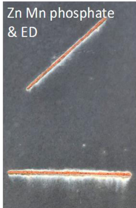
August 2018, 3 weeks outdoor exposure, west coast of Sweden RISE weathering test lab, Bohus Malmön Sweden, steel plates 45 degrees from vertical
